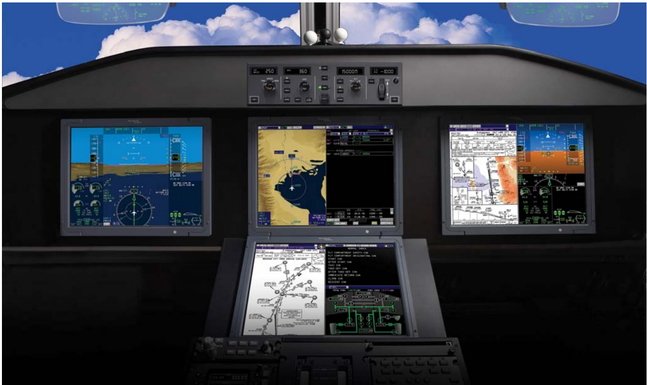
Figure 3 – Pilot Display Panels
